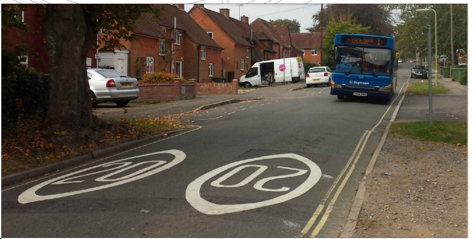
Example of 20 mph roundel arrangement used to maintain slower traffic speeds
